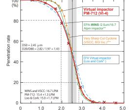
Comparison virtual-impactor with main PM<sub>2.5</sub> separator
